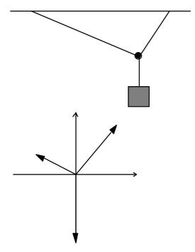
A block of weight W is suspended by strings (a). Consider the knot at the junction of the three strings to be the body. A free-body diagram shows all the forces acting on the knot (b). The strings are assumed to be weightless. The body remains at rest under the action of the three forces. Suppose we are given the magnitude of one of these forces. How can we find the magnitudes of the other forces?
